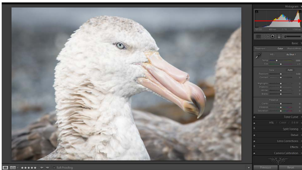
Above: Original capture without processing - note how the histogram is close to the right hand (brightest tone) end of the graph.
